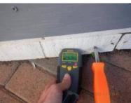
[CR] There was evidence of moisture intrusion to the shed. We recommend locating and correcting the source and any damaged materials.
